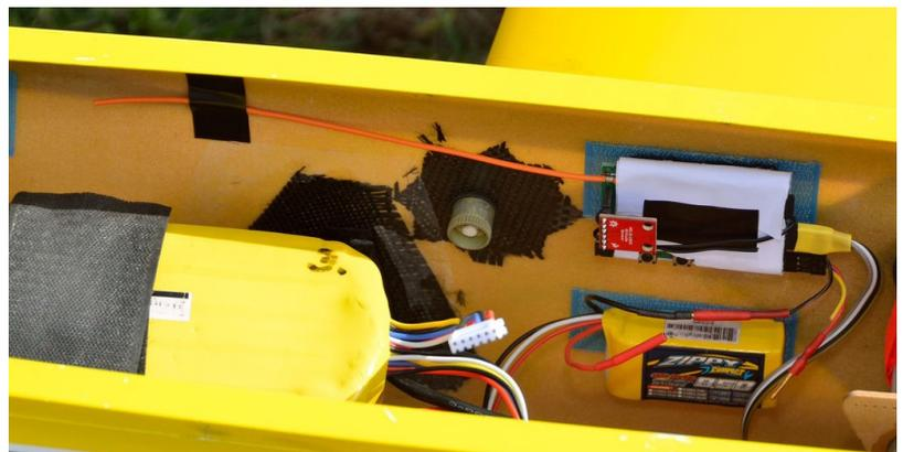
The optimum position for the RX is such arrangement to the receiving antenna is pointing parallel to the flight zone.
